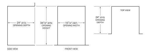
Dimensions in parentheses are in millimeters unless otherwise specified.
